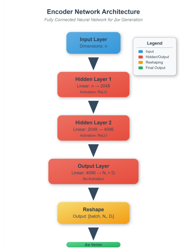
Figure 2: Encoder network architecture for StyleGAN2-Stego, mapping the binary secret message into a perturbation vector \Delta w aligned with the StyleGAN2-ADA latent space
