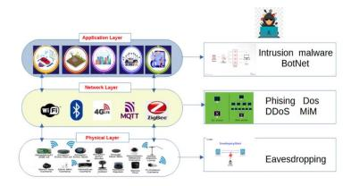
**Figure 1:** Architecture of IoT layers & Attacks [10]
