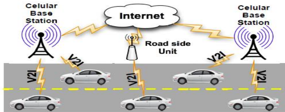
Figure 1: Vehicle-to-Infrastructure (V2I) communication. [11]
